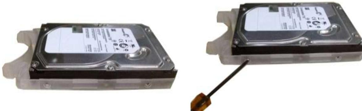
① Line up the handle to the HDD side (without the interface) ② Use the screwdriver to fix the handle on the HDD.
