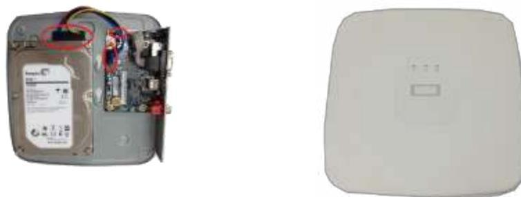
④ Connect the HDD cable and power cable to the HDD and the mainboard respectively. ⑤ Put the cover back and then fix the screws of the rear panel. The installation is complete.
