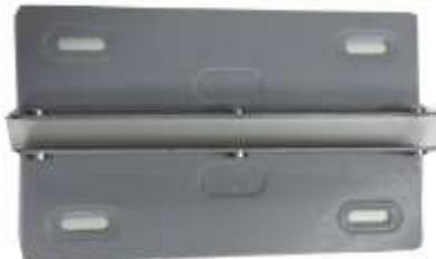
① Open top cover and then remove the HDD bracket
