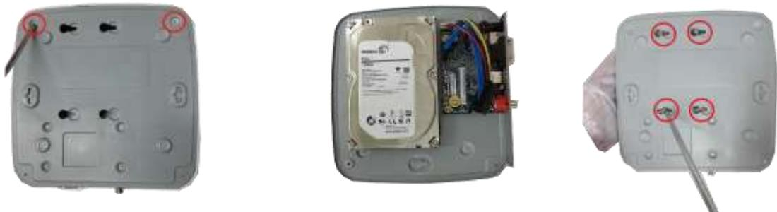
①. Loosen the screws of the bottom of the chassis. ② Place the HDD in accordance with the four holes in the bottom. ③ Turn the device upside down and then secure the screws firmly.
