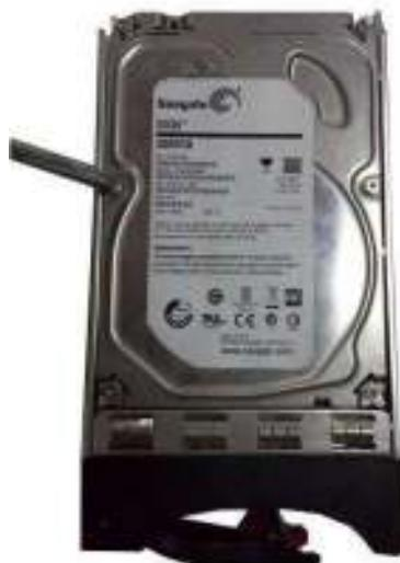
① Use four screws to secure the HDD.
