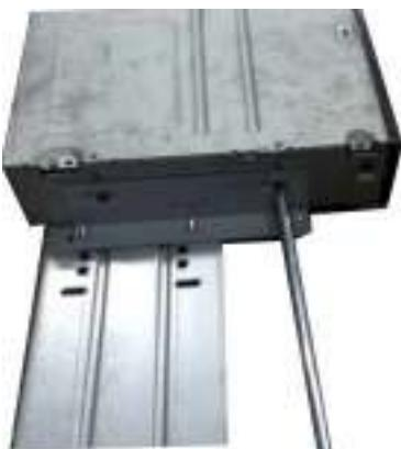
⑤ Install SATA burner. Line up the SATA burner to the hole positions.
