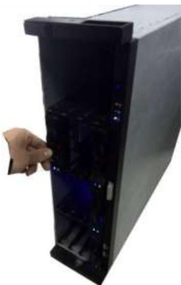
③Please pull the handle up when you are inputting the HDD box in case the handle collides with the front panel
