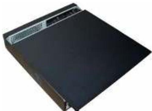
① ①Use the screwdriver to loose the screws of the rear panel and then remove the front cover.
