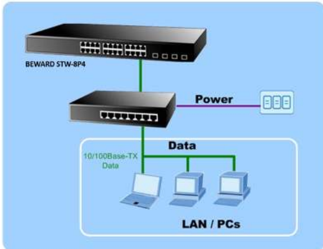
Figure 2-7 End node or Switch connection
